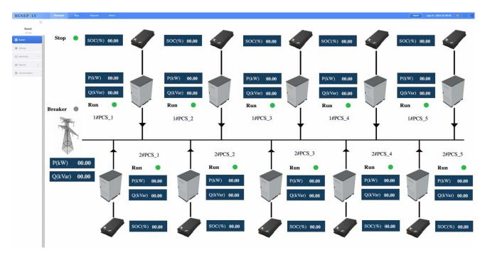
**Operation settings page:** The microgrid supports three operation modes: manual mode, automatic mode, and proxy mode.
